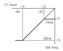
▶ 16 ~ 110: Setting input range and corresponding frequency to 0 ~ +10V V1 input voltage
