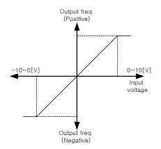
▶ I 2 ~ I 5: Setting input range and corresponding frequency to -10V ~ 0V V1 input voltage Ex) when minimum (-) input voltage is -2V with corresponding frequency 10Hz and Max voltage is -8V with run freq. 50Hz.
