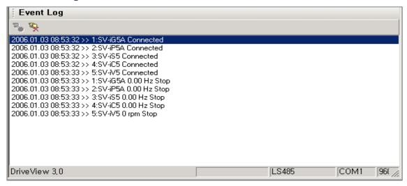
After starting DriveView 3.3, this window can display max. 200 of operation status, connection status, and fault history of inverters connected in communication network.
