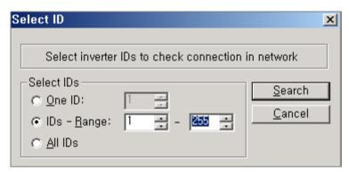
This searches the inverters connected via communication network, and shows main status of inverters on 'Select ID'.
