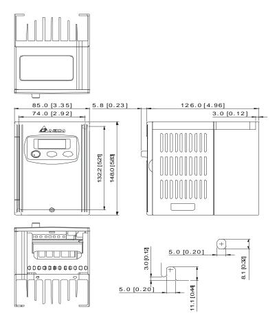
Frame S1: VFD004S43B, VFD007S43B
