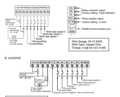
Wire Gauge: 24-16 AWG Wire Type: Copper Only Torque: 2 kgf-cm (1.7 in-lbf)
