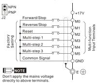
17 Vdc +17V Forward/Stop M0 Reverse/Stop nput Terminals M1 Multi-function Factory Setting Reset M2 Multi-step 1 M3 Multi-step 2 M4 Multi-step 3 M5 GND Е 🕀
