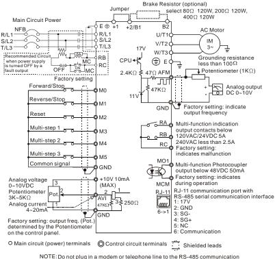
OTE: Do not plug in a modem or telephone line to the RS-485 communicatio port, permanent damage may result. Pins 1&2 are the power sources for the optional copy keypad and should not be used while using RS-485 communication.
