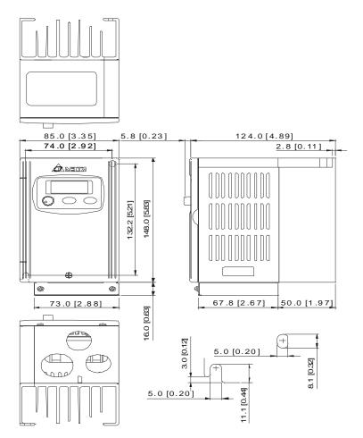
Frame S1: VFD004S43A, VFD004S43E, VFD007S43A, VFD007S43E
