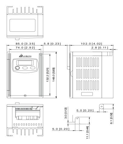
Frame S1: VFD004S11B, VFD004S21B
