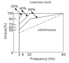
E. If 100% continuous torque is required at low speed, it may be necessary to use a special inverter duty motor.
