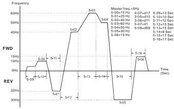
\* The calculation of time for Pr.5-11, Pr.5-12, Pr.5-15 and Pr.5-16 should be carefully planned.
