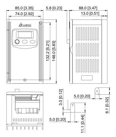
Frame S1: VFD002S11B, VFD002S21B
