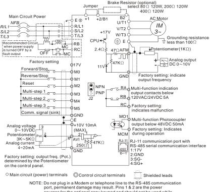
sources for the optional copy keypad and should not be used while using RS-485 communication.
