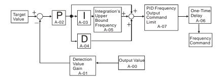
If the input range of sensor is 0~SI\_max, output range is SO\_min~SO\_max and then
