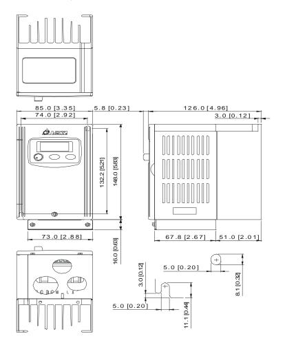
Frame S1: VFD002S21E, VFD004S21E, VFD007S21E, VFD015S23D
