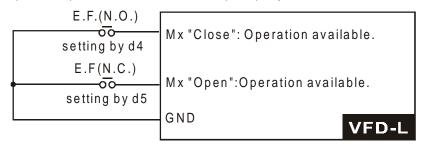
When an External Fault input signal is received, the AC drive will stop all output and display "E.F." on Digital Keypad, the motor will free run. Normal operation can resume after the External Fault is cleared and the AC drive is reset.
