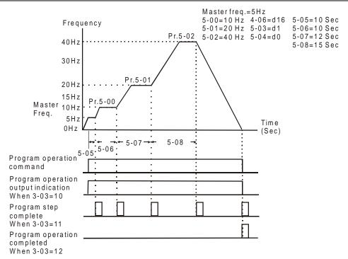
Note: The above diagram shows one complete PLC cycle. To restart the cycle, turn the PLC program off and then back on.
