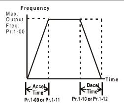
$Actual\ Accel/Decel\ Time = \frac{Accel/Decel\ Time\ x(Master\ Freq.-Min.Output\ Freq.)}{Max.\ Output\ Freq.}$
