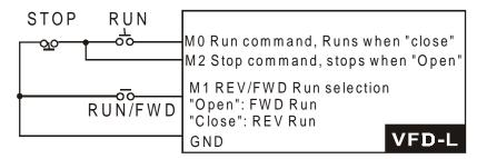
Note: When value d3 is selected for Pr. 4-04, this will over ride any value entered in Pr.4-05, since Pr.4-05 must be used for three wire control as shown above.
