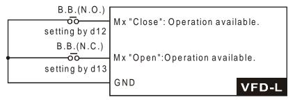
**Note:** When a Base-Block signal is received, the AC drive will stop all output and the motor will free run. When base block control is deactivated, the AC drive will start its speed search function and synchronize with the motor speed, and then accelerate to Master Frequency.
