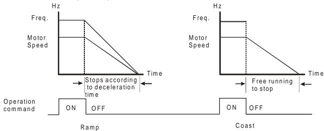
Note: The motor stop method is usually determined by the characteristics of the motor load and frequency of stops.
