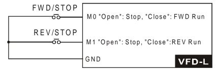
d2: Two wire operation: Restrict to Pr. 4-04 and external terminals M0, M1.
