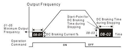
NOTE: 1. DC Braking during Start-up is used for loads that may move before AC drive starts, such as fans and pumps. These loads may also be moving in the wrong direction. Under such circumstances, DC Braking can be executed to hold the load in position before applying a forward motion.
