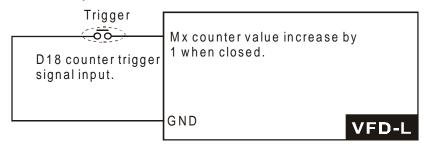
Note: The Counter Trigger input can be connected to an external Pulse Signal Generator to count a processing step or unit of material. See the diagram below.
