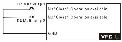
These three inputs select the multi-step speeds defined by Pr.5-00 to Pr.5-02 as shown in the following diagram. Pr.5-05 to Pr.5-8 can also control output timing by programming the AC drive's internal PLC function.
