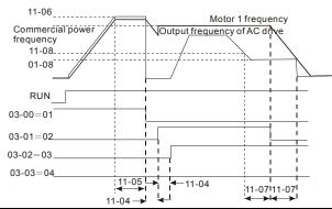
11 - 06 Motor Switch Frequency during Fixed Amount Circulation
