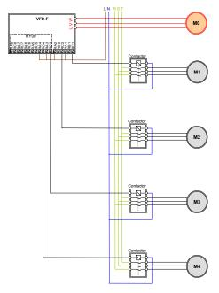
When this parameter isn't set to 00, 03-00 to 03-07 multi-function terminals will automatically set the corresponding output motor.
