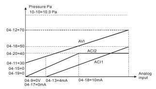
When analog input current of ACI1/ACI2 is lower than Pr.04-13/Pr.04-17, EF warning will pup-up.
