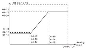
Example: Using the AVI(0~10V) as the target source and ACI1(4~20mA corresponds to 0~5Pa) and ACI2(0~10mA corresponds to 0~4Pa) as the feedback location for a pressure sensor connected. If your target value is between 3~7Pa (Set Pr.10-01 to 10, other parameters settings refer Pr.10-01 to set as shown in the following diagram and then setting the PID feedback relative parameters.) If setting AVI to 7.5V, pressure sum of ACI1 and ACI2 could be controlled at 6Pa.
