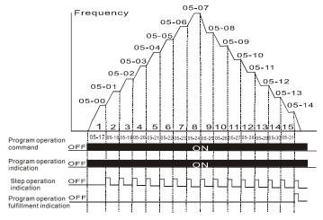
Note: The above diagram shows one complete PLC cycle. To restart the cycle, turn the PLC program off and on again.
