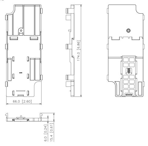
This DIN rail (MKEL-DRA) is only for frame A. For frame B, it is shipped with DIN rail (MKEL-DRB). Refer to chapter 1.3 for VFD-EL dimension.
