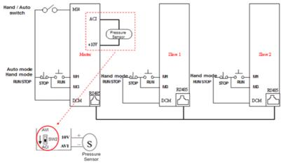
Wiring of the pressure sensor:
