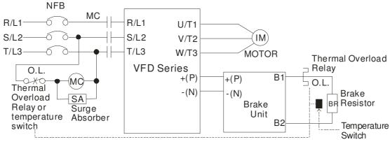
Note 1: When using the AC drive with DC reactor, please refer to wiring diagram in the AC drive user manual for the wiring of terminal +(P) of Brake unit.
