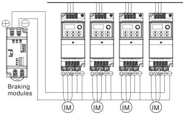
For frame A and B, terminal + (-) is connected to the terminal + (-) of the braking module.
