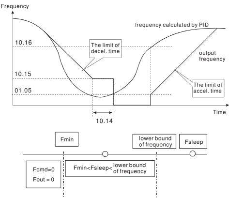
When output frequency ≤ sleep frequency and time > detection time, it will go in sleep mode.
