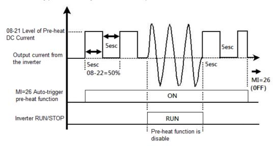
The figure below shows the sequential relationship, when MI=26 pre-heat is disabled, pre-heat DC current is enabled and cycle time is 50%. When the motor drive is stopped, the pre-heat function will start to output DC current continuously.
