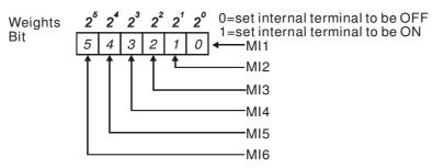
For example, if setting MI3, MI5 and MI6 to be ON, Pr.04.28 should be set to bit5X2<sup>5</sup>+bit4X2<sup>4</sup>+bit2X2<sup>2</sup>= 1X2<sup>5</sup>+1X2<sup>4</sup>+1X2<sup>2</sup>= 32+16+4=52 as shown in the following.
