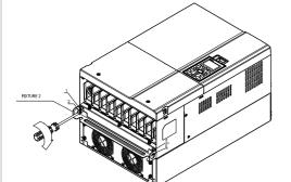
5. Fasten 4 screws (as shown in the following figure). Screw torque: 24~26kg-cm (20.8~22.6lb-in).
