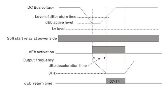
**IF NOTE** If Pr07-14 is set to 0, then a STOP command will be given. Besides the motor drive will not accelerate to reach the frequency before dEb even if the power is on again. If Pr07-14 is not set to 0, a command of zero speed will be given and wait for the power on.
