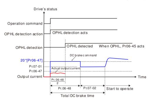
□ Status 4: Motor drive is in stop; Pr06-48≠0 ; Pr07-02=0
