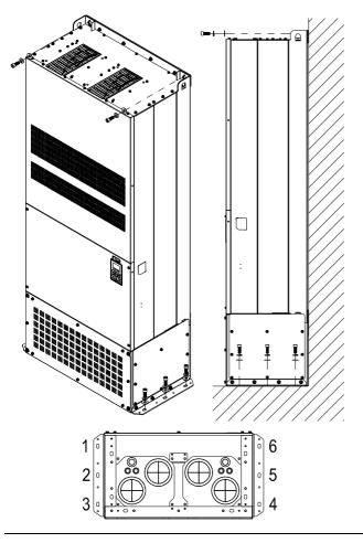
Secure the drive from the external. Screw: M12\*8 Torque: 340-420kg-cm [295.1-364.6lb-in.]
