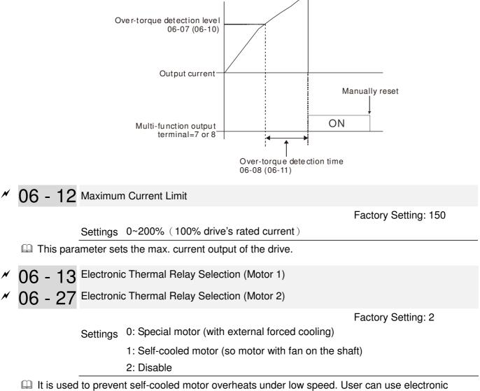
thermal relay to limit driver's output power.
