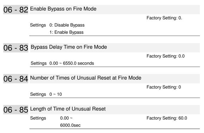
The settings of Pr06-82 to Pr06-85 decide if switch motors to operating under mains electricity.
