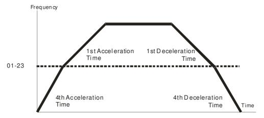
1st/4th Acceleration/Deceleration Frequency Switching
