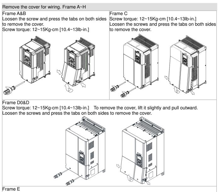
Screw torque: 12~15Kg-cm [10.4~13lb-in.] To remove the cover, lift it slightly and pull outward.
