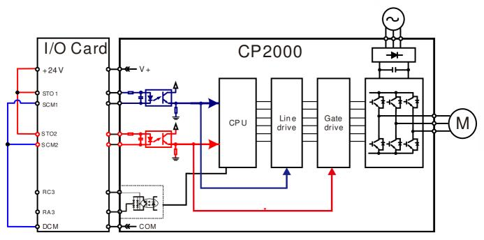
20-3-3 The control loop wiring diagram:
