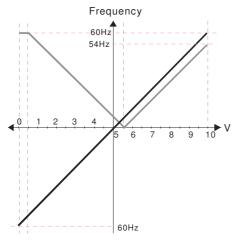
$\label{eq:Pr.00-21=0} \mbox{(Digital keypad control and d run in FWD direction)} \\ \mbox{Pr.03-05 Analog Positive Voltage Input Bias (AVI2) = 10\% }$
