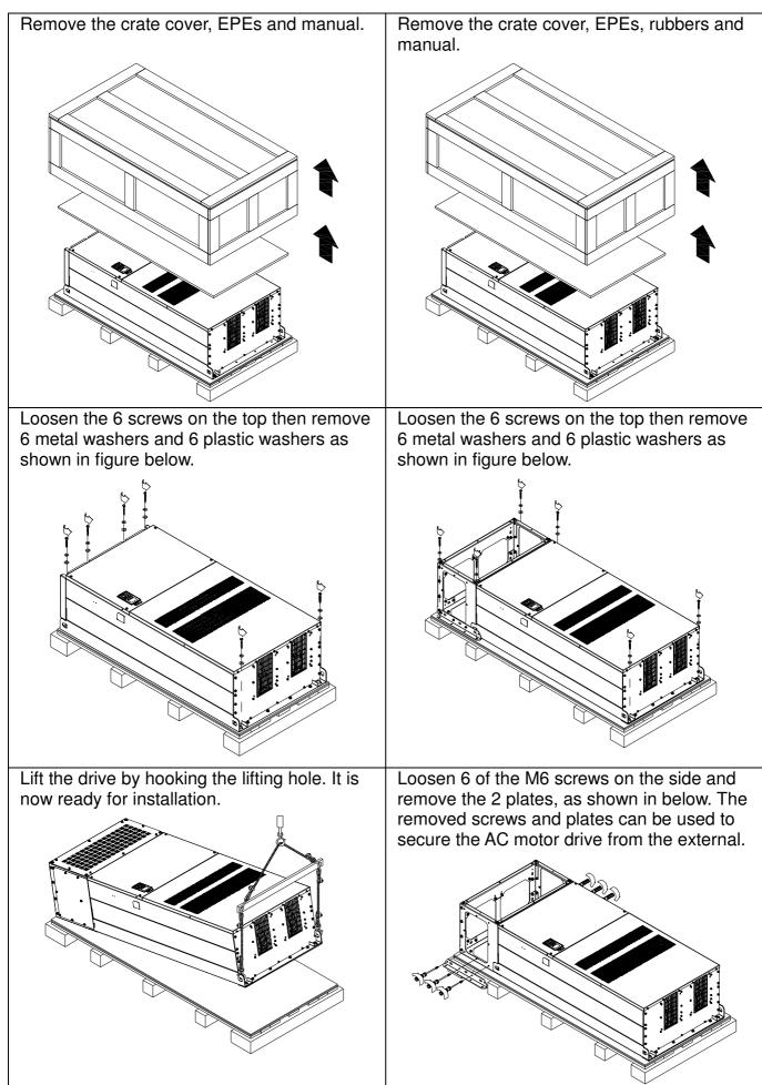
Secure the drive from the external. (Skip to the next step if it is not necessary in your case)
