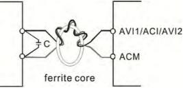
Wind each wires 3 times or more around the core
