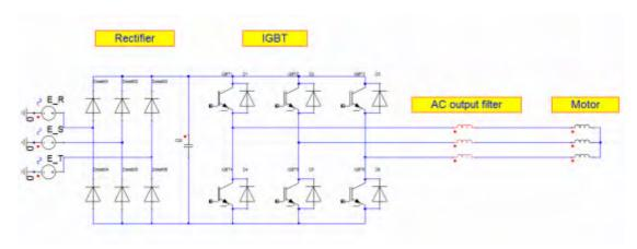
AC output reactor setup
