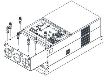
Place the cover back to the top and fasten the screws (as shown in the figure). Screw torque:  $12 \sim 15$ kg-cm ( $10.4 \sim 13$ lb-in).
