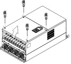
Remove the top cover and loosen the screws. M5 Screw torque: 24~26kg-cm (20.8~22.6lb-in) M8 Screw torque: 100~120kg-cm (86.7~104.1lb-in)
