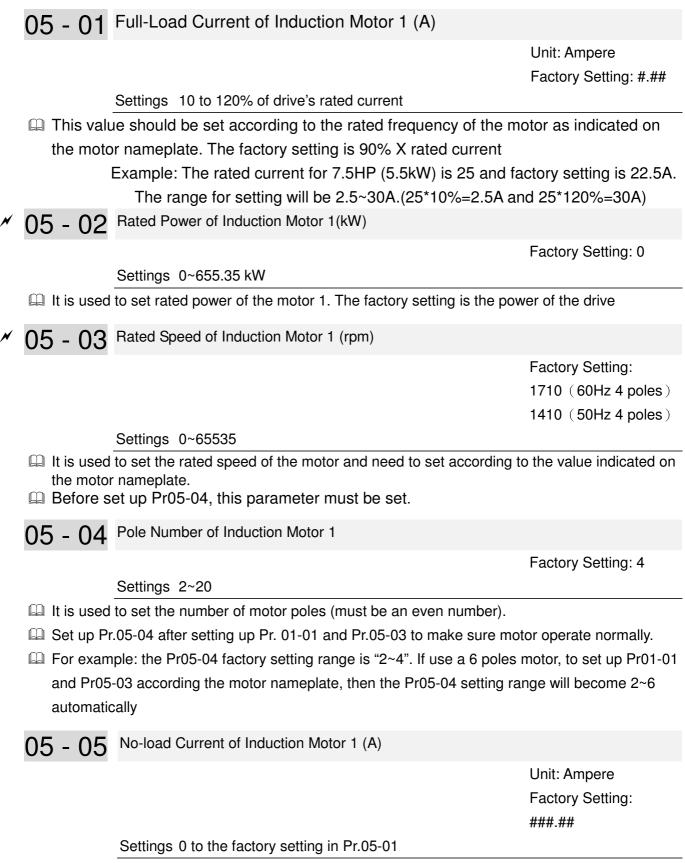
The factory setting is 40% motor rated current.
