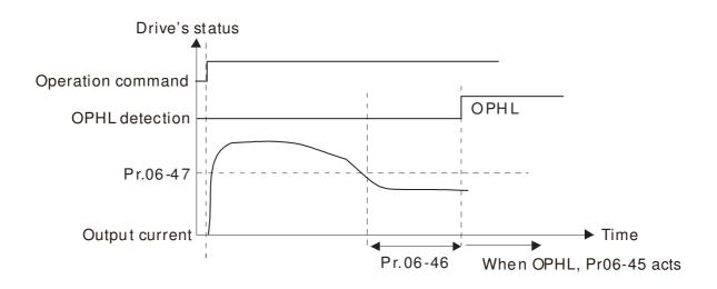
□ Status 2 : Motor drive is in stop; Pr06-48=0 ; Pr07-02≠0
