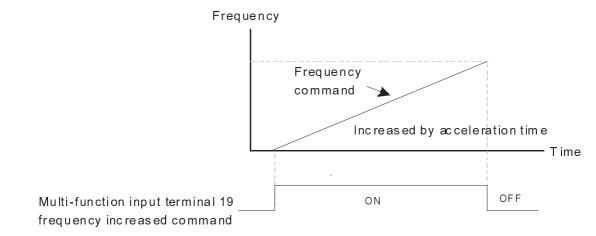
Pr.02-09 set to 1: use multi-function input terminal ON/OFF to increase/decrease the frequency command(F) according to the setting of Pr.02.10(0.001~1.000Hz/ms).
