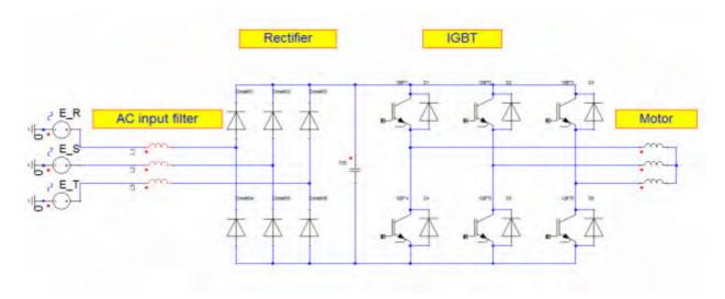
AC input reactor setup
