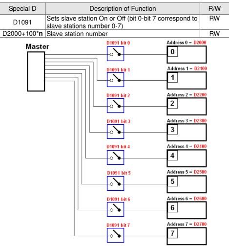
If slave devices have a slow start-up, the master can delay for a short time before performing slave station configuration; this time delay can be set via D1092.
