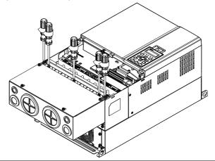
4. Fasten the 2 screws shown in the following figure. Screw torque: 12~15kg-cm (10.4~13 lb-in)
