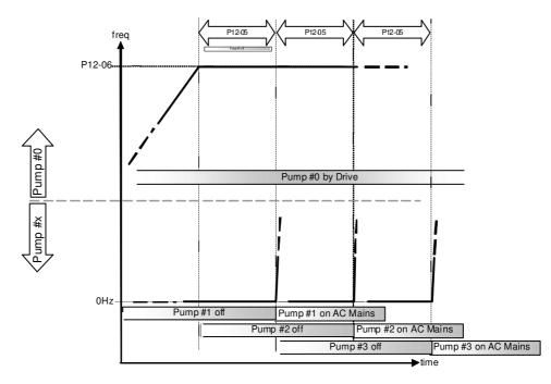
Diagram 12-9: Sequence of switching motors at Fixed quantity control with PID – Increasing Demand
