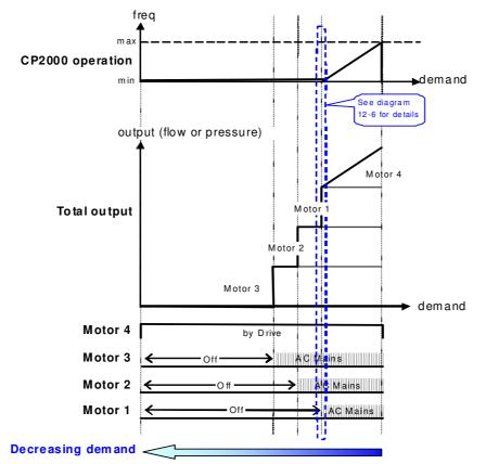
Diagram 12-5: Sequence of switching motors at Fixed quantity circulation with PID – Decreasing Demands
