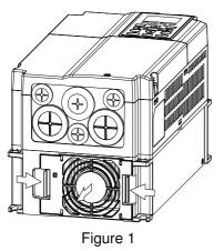
2. Disconnect the power terminal before removing the fan.
