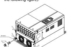
Fasten 4 screws (as shown in the following figure). 3. Screw torque: 30~32kg-cm (26.0~27.8lb-in).
