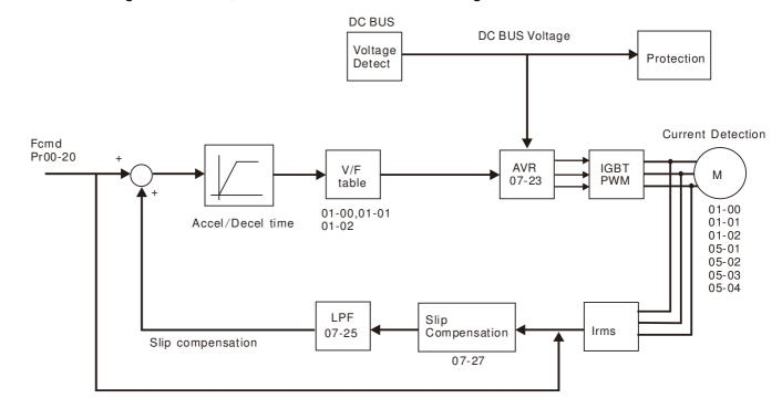
When setting Pr.00-11 to 2, the sensorless vector control diagram is shown as follows.
