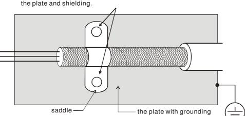
Remove any paint on metal saddle for good ground contact with
