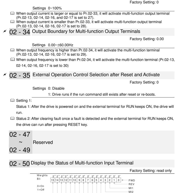
For Example: If Pr.02-50 displays 0034h (Hex), i.e. the value is 52, and 110100 (binary). It means MI1, MI3 and MI4 are active.
