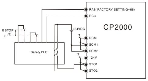
\*1: factory short circuit of DCM-SCM1-SCM2. To use the Safety function, please remove this short circuit
