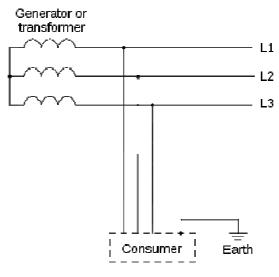
motor drive or the AC servo motor drive is connected to an IT system.
