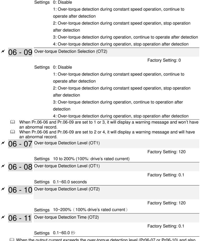
When the output current exceeds the over-torque detection level (Pr06-07 or Pr06-10) and also exceeds Pr06-08 or Pr06-11, the over torque detection will follow the setting of Pr06-06 and Pr06-09.
