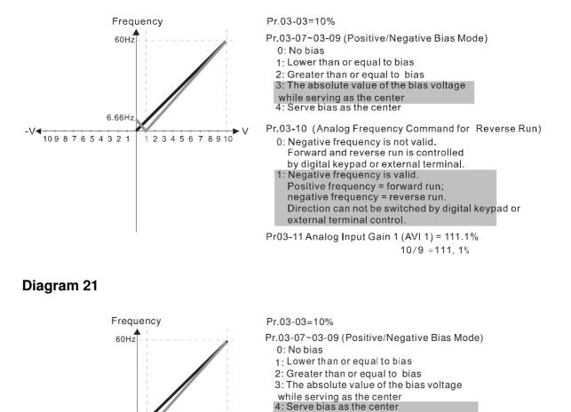
Pr.03-10 (Analog Frequency Command for Reverse Run)
