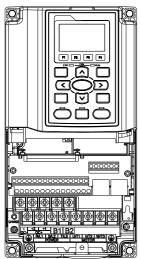
Main circuit terminals: R/L1, S/L2, T/L3, U/T1, V/T2, W/T3, , B1, B2, +1, +2, -
