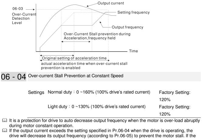
drive will decrease its output frequency (according to Pr.06-05) to prevent the motor stall. If the output current is lower than the setting specified in Pr.06-04, the drive will accelerate (according to Pr.06-05) again to catch up with the set frequency command value.
