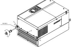
Fasten 5 screws (as shown in the following figure). 6. Screw torque: 24~26kg-cm (20.8~22.6lb-in).
