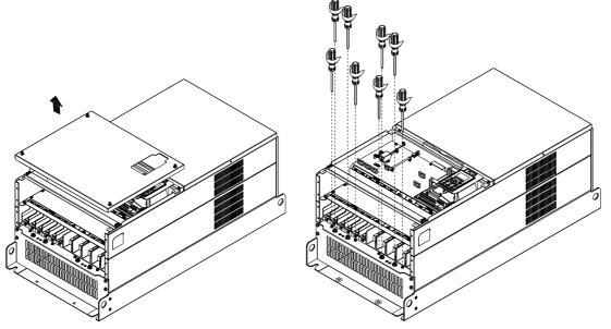
Install the conduit box by fastening all the screws shown in the following figure. M5 Screw torque: 24~26kg-cm (20.8~22.6lb-in) M8 Screw torque: 100~120kg-cm (86.7~104.1lb-in)
