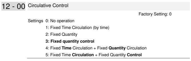
In this mode, CP2000 can control up to 8 motors at a time. The total number of the motors can be determined by Pr.12-01. In accordance with the Fixed Time Circulation of Pr12-02, you can adjust the switching time between Start/Stop of each motor. That means when an operating motor reaches the time setting of Pr12-02, CP2000 will stop that motor. Then after the delay time setting of Pr12-03, next motor will start operating. See diagram below.
