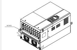
7. Place 4 screws (M10) through Fixture 1&2 and the plate then fasten the screws. (as shown in the following figure) Frame D0/D M10\*4 Screw torque: 200~240kg-cm (173.6~208.3lb-in).
