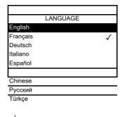
Display after the graphic display terminal has been powered up for the first time. Select the language and press ENT.
