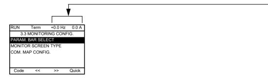
**[PARAM. BAR SELECT]**: Selection of 1 to 2 parameters displayed on the top line (the first 2 cannot be modified).
