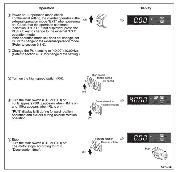
Fig. 5-24: Operate the inverter by using external signals
