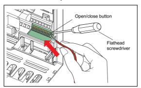
Fig. 3-11: Connection of a stranded wire
