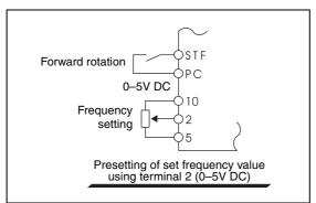
Fig. 6-80: Frequency setting by voltage 0–5V DC
