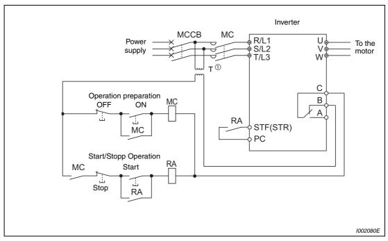
Fig. 3-23: Example for connection of an inverter
