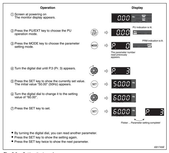
Fig. 5-2: Setting the base frequency
