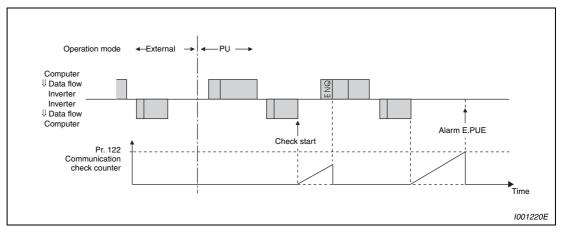
Fig. 6-105: Signal loss detection
