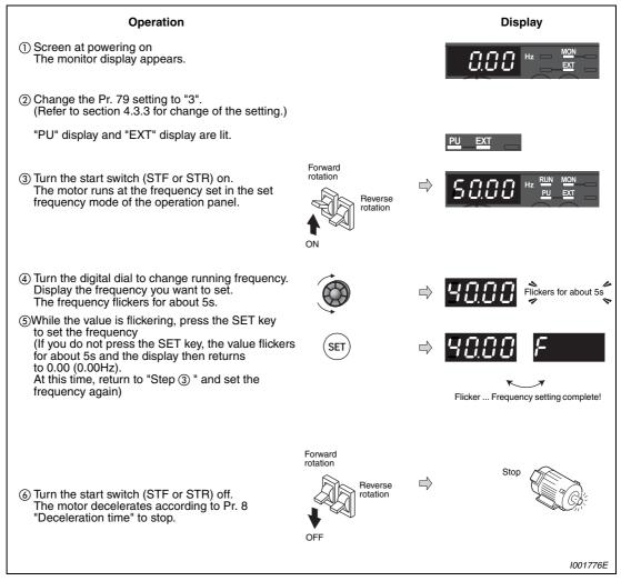
Fig. 5-21: Operate the inverter by using external signals
