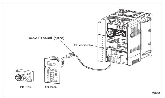
Fig. 3-22: Connecting a parameter unit using a connection cable
