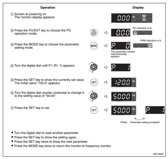
Fig. 4-12: Setting the maximum output frequency
