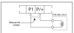
Fig. 3-34: Connection of a DC reactor
