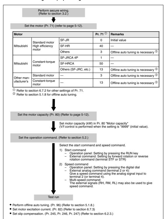
Fig. 6-2: Selection method of general-purpose magnetic flux vector control
