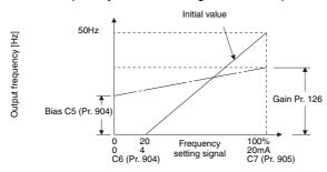
As other adjustment methods of frequency setting current gain, there are methods to adjust with a current flowing in the terminals 4-5 and adjust at any point without a current flowing. (Refer to section 6.15.3 for the setting method of calibration parameter C7.)
