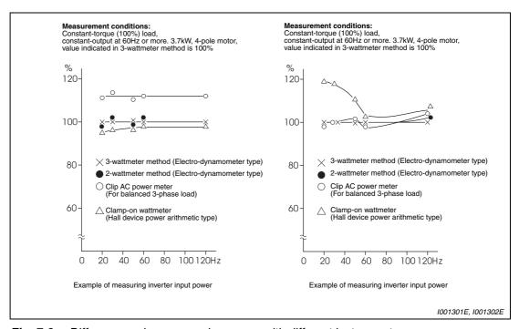
Fig. 7-8: Differences when measuring power with different instruments
