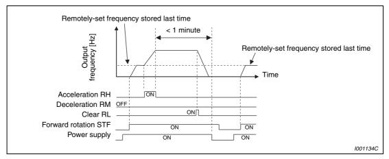
Fig. 6-25: Outputting the remotely-set frequency stored last time
