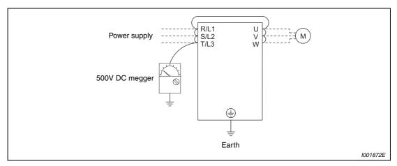
Fig. 8-7: Insulation resistance test
