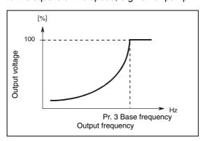
Fig. 6-13: Variable-torque load
