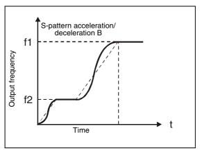
**Fig. 6-32:** Characteristic for parameter 29 = 2
