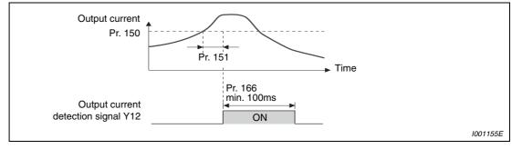
**Abb. 6-55:** Output current detection (Pr. 166 ≠ 9999, Pr. 167 = 0)
