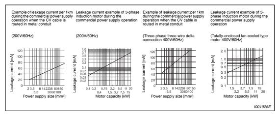
Fig. 3-37: Leakage currents
