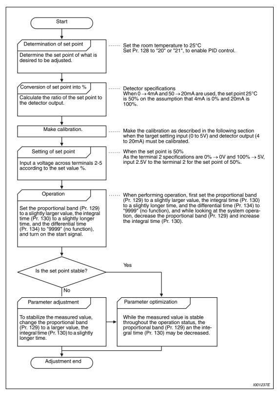
Fig. 6-129: Calibration example
