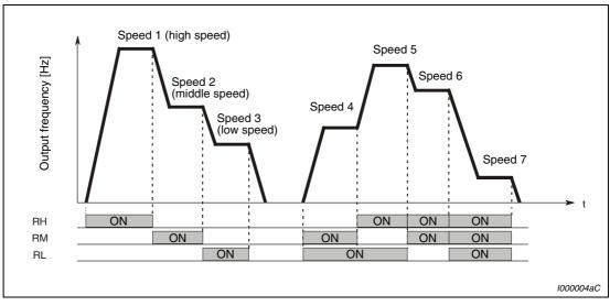
Fig. 5-14: Multi-speed selection by external terminals
