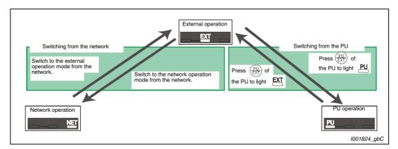
Fig. 6-90: Switching the operation mode when Pr. 340 = 0 or 1
