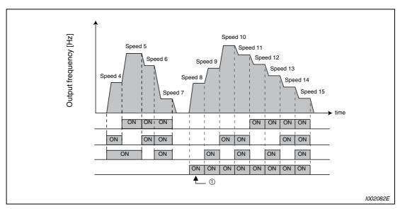
Fig. 6-16: Multi-speed selection by external terminals
