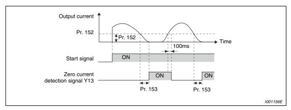
Fig. 6-56: Zero current detection
