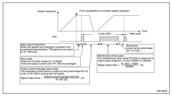
Fig. 6-143: Output of the pulse signal Y93
