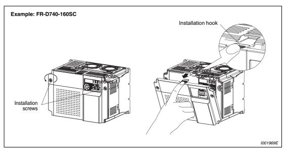
Fig. 2-3: Removal of the front cover
