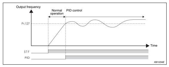
Fig. 6-126: Automatic switchover to PID control
