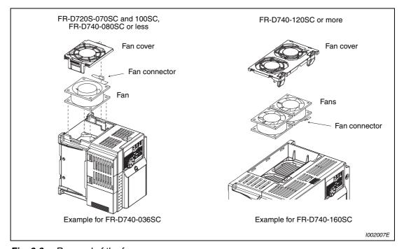
Fig. 8-3: Removal of the fan
