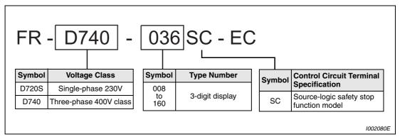
Fig. 1-1: Inverter type FR-D700 SC EC
