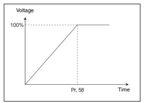
Fig. 6-70: Voltage rise at automatic restart
