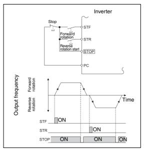
**Fig. 6-49:** 3-wire type connection (Pr. 250 = 9999)
