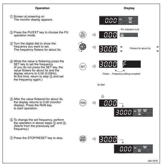
Fig. 5-11: Frequency setting with the digital dial
