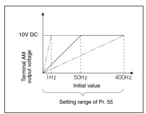
Fig. 6-63: Frequency monitoring reference
