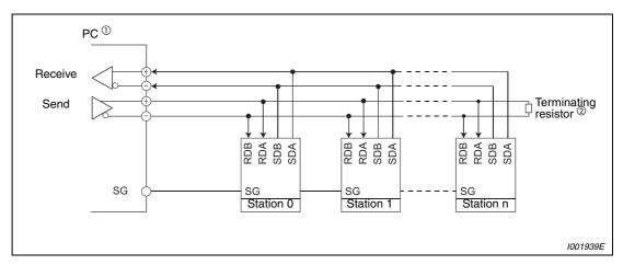
Fig. 6-102: Connection to several inverter
