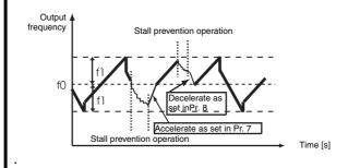
When the value of amplitude inversion compensation amount (Pr. 594, Pr. 595) is too large, pattern operation as set is not performed due to overvoltage shut-off and stall prevention.
