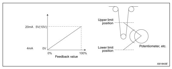
Fig. 6-135: Dancer roller position detection signal adjustment
