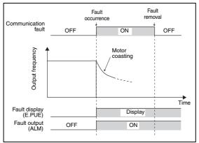
Fig. 6-106: Operation when Pr. 502 setting is "0" (initial value)
