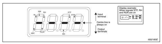
Fig. 6-62: Displaying the signal states of the I/O terminals
