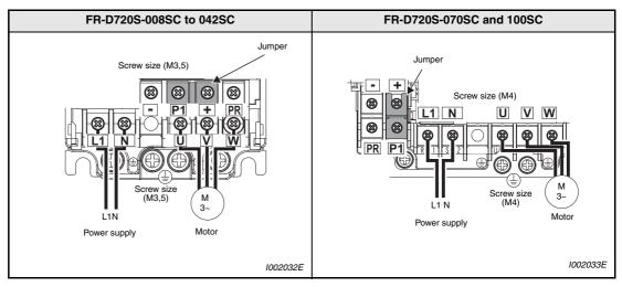
Tab. 3-3: Terminal layout and wiring
