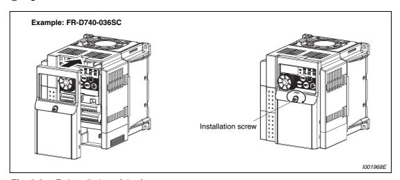
Fig. 2-2: Reinstallation of the front cover
