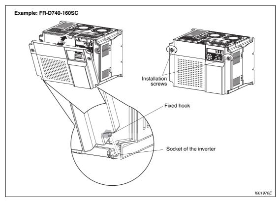
Fig. 2-4: Reinstallation of the front cover
