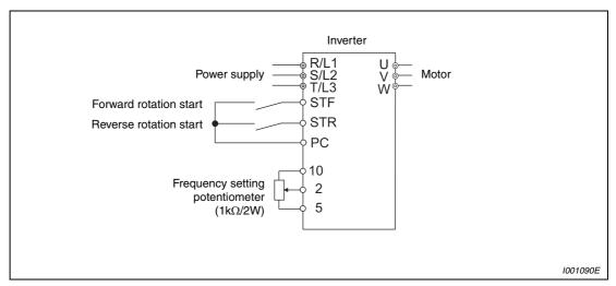
Fig. 5-25: Frequency setting by analog voltage input
