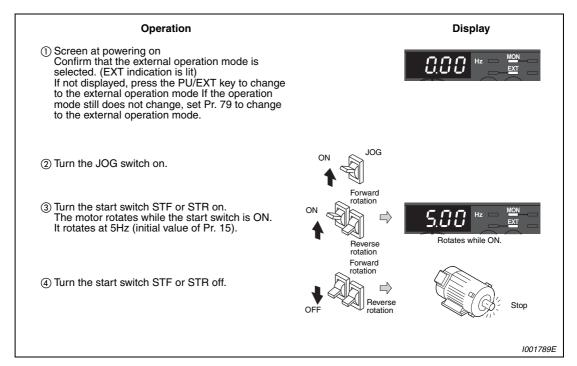
Fig. 6-20: Jog operation in the external operation mode
