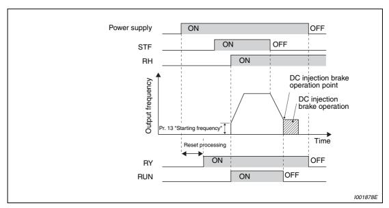
Fig. 4-3: Ready status and motor running
