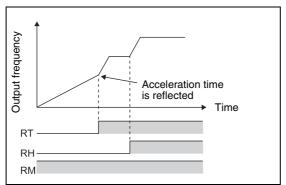
**Fig. 6-46:**Second acceleration/deceleration time example
