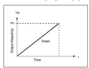
Fig. 6-30: Characteristic for parameter 29 = 0
