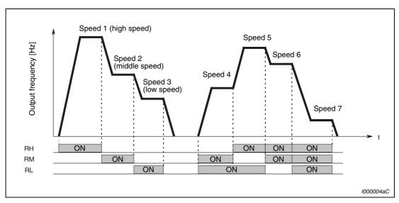
Fig. 5-23: Multi-speed selection by external terminals
