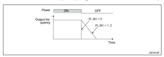
Fig. 6-71: Parameters for stop selection at power failure
