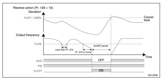
Fig. 6-127: PID output suspension function (SLEEP function)
