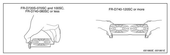
Fig. 8-2: Removal of the fan cover
