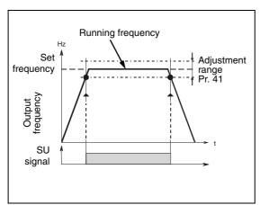
Fig. 6-53: Output of the SU signal
