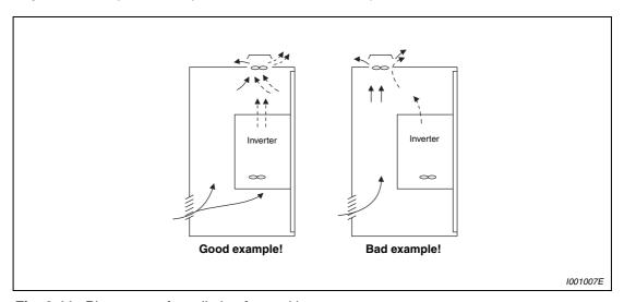
Fig. 2-11: Placement of ventilation fan and inverter
