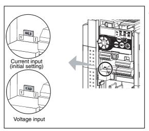
Fig. 6-79: Voltage/current input switch
