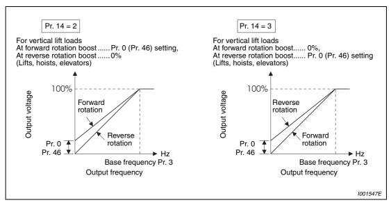
Fig. 6-14: Characteristic with manual torque boost
