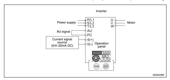
Fig. 5-18: Frequency setting by analog current input
