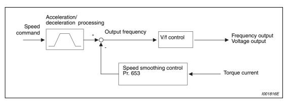
Fig. 6-78: Control block diagram of the speed smoothing control
