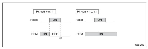
Fig. 6-59: Signal condition during a reset
