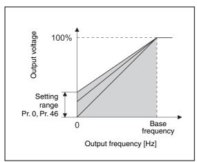
Fig. 5-3: Relation between output frequency and output voltage
