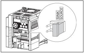
Fig. 3-18: Changing the control logic
