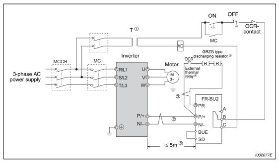
Fig. 3-29: Connection with the brake unit FR-BU2
