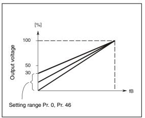
Fig. 6-1: Relationship between output frequency and output voltage
