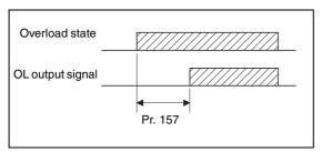
Fig. 6-5: Output of the OL signal
