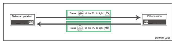
Fig. 6-91: Switching the operation mode when Pr. 340 = 10
