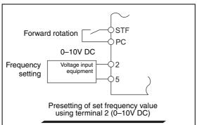
Fig. 6-81: Frequency setting by voltage 0–10V DC
