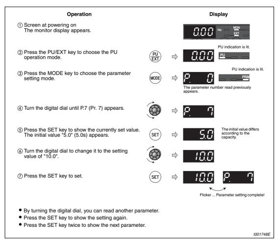
Fig. 5-8: Setting the acceleration time
