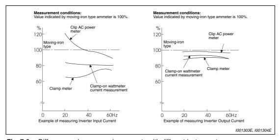
Fig. 7-9: Differences when measuring currents with different instruments
