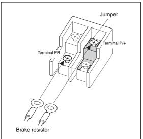
Fig. 3-25: Connection of a brake resistor to the terminals P/+ and PR for the inverters FR-D720S-070SC and 100SC and FR-D740-012SC to FR-D740-080SC
