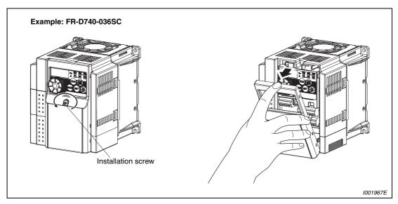
Fig. 2-1: Removal of the front cover
