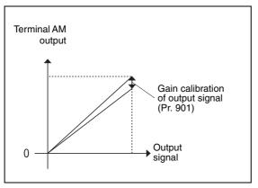
Fig. 6-66: Terminal AM gain calibration
