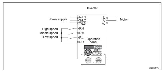
Fig. 5-13: Use switches to give the frequency command
