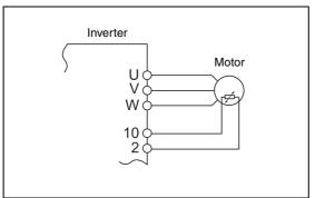
Fig. 6-37: PTC thermistor input connection
