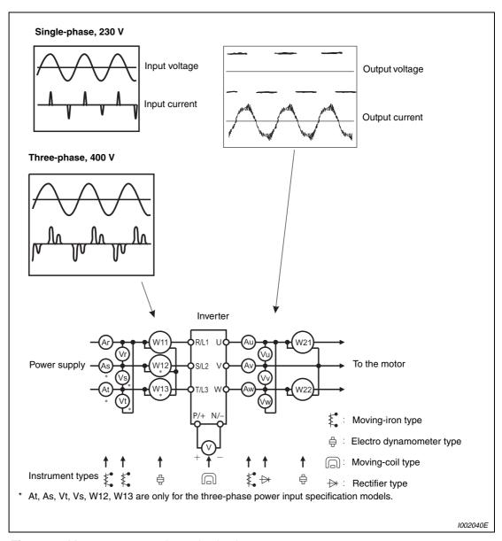
Fig. 7-7: Measurements at the main circuit
