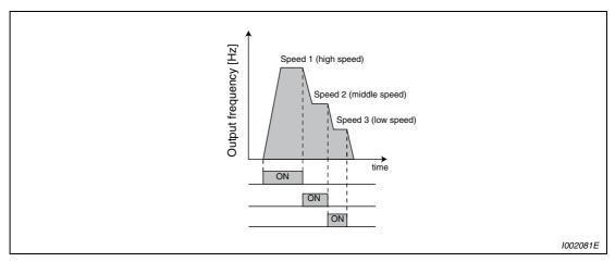
Fig. 6-15: Multi-speed selection by external terminals
