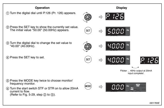
Fig. 5-30: Change the frequency of the maximum analog value
