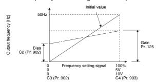
As other adjustment methods of frequency setting voltage gain, there are methods to adjust with a voltage applied to across terminals 2-5 and adjust at any point without a voltage applied. (Refer to section 6.15.3 for the setting method of calibration parameter C4.)
