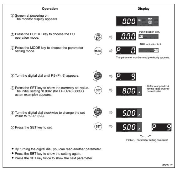
Fig. 5-1: Setting of the electronic thermal O/L relay
