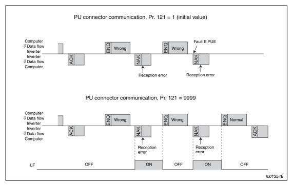
Fig. 6-104: Data transmission error
