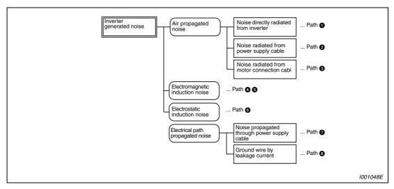
Fig. 3-38: Noise propagation
