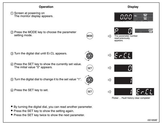
Fig. 7-6: Clearing the fault history
