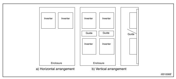
Fig. 2-10: Arrangement of multiple inverters
