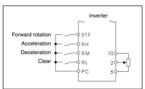
Fig. 6-23: Connection diagram for remote setting
