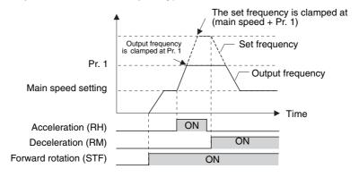
When the acceleration or deceleration signal switches ON, acceleration/deceleration time is as set in Pr. 44 and Pr. 45. Note that when the time set in Pr. 7 or Pr. 8 is longer than the time set in Pr. 44 or Pr. 45, the acceleration/deceleration time is as set in Pr. 7 or Pr. 8. (when RT signal is OFF). When the RT signal is ON, acceleration/deceleration is made in the time set in Pr. 44 and Pr. 45, regardless of the Pr. 7 or Pr. 8 setting.
