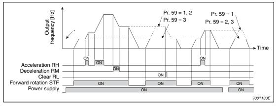
Fig. 6-24: Example of the remote setting function
