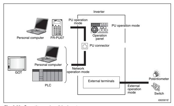
Fig. 6-89: Operation modes of the inverter
