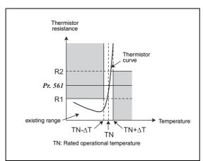
Fig. 6-38: PTC thermistor characteristics
