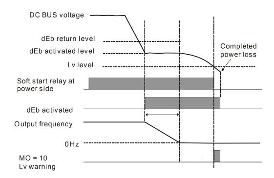
• Situation 4: Power supply unexpected shut down / power loss
