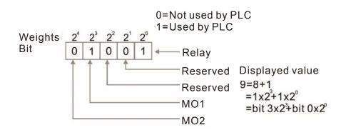
**B2-54** Display Memory of Frequency Command Used by External Terminal
