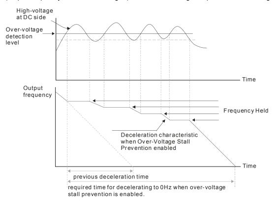
When Pr. 06-02 is set to 1: When use smart over-voltage stall prevention during deceleration, the drive will maintain DC bus voltage when decelerating and prevent the drive from OV.
