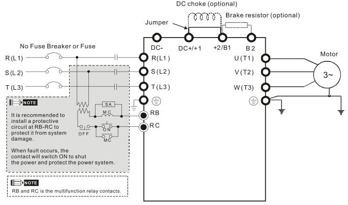
Wiring of DC reactor
