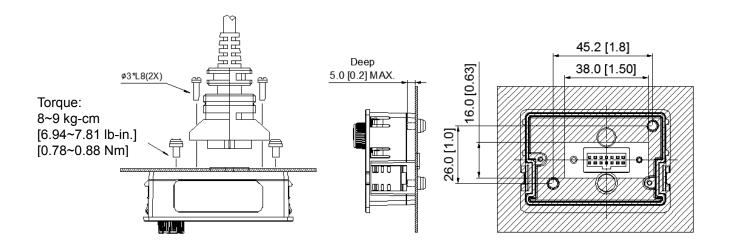
**Method 2**: Mounting through a plate (unit: mm [inch]) Thickness = 1.2 [0.05] or 2.0 [0.08]
