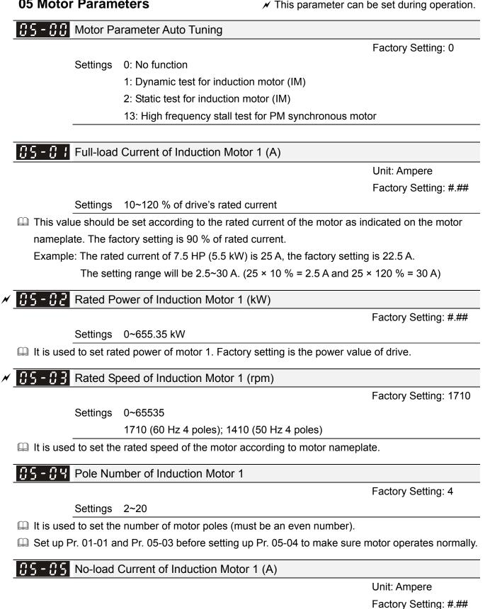
Definition The factory setting is 40 % of the motor rated current.
