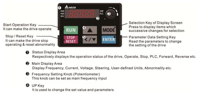
LEFT/ DOWN Key It is used to change the set value and parameters (use left key by long pressing MODE key)
