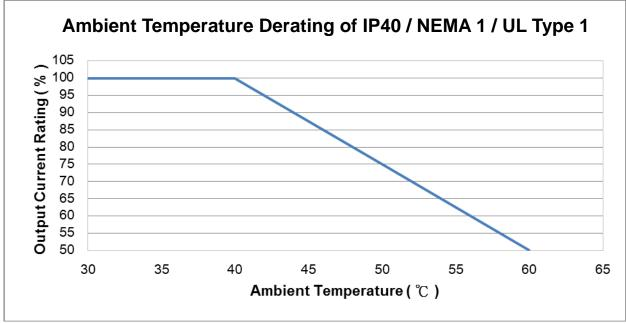
At rated current the ambient temperature is  $-10^{\circ}$ C ~  $+40^{\circ}$ C. Over 40°C the rated current has to be decreased 2.5%/°C up to 60°C.
