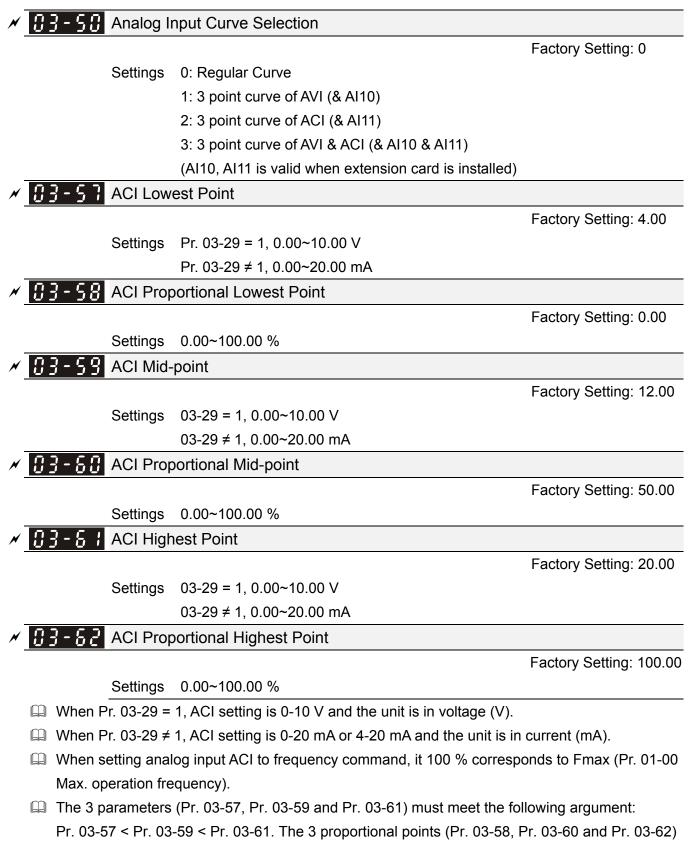
doesn't have any limit. Between two points is a linear calculation.
