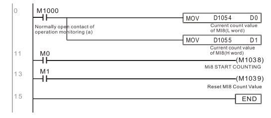
% When the PLC program defines MI7 for use as a high-speed counter, and also for use in PLC procedures, it must be written to M1038 or M1039, and the original MI8 functions will be disabled.
