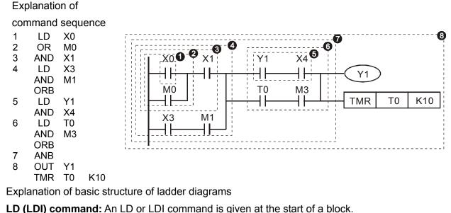
LD command LD command AND Block **OR Block** LDP and LDF have this command structure, but there are differences in their action state. LDP, LDF only act at the rising or falling edge of a conducting contact. (See figure below): Rising-edge Falling-edge XΟ XΟ Time ┨╁┠ Time OFF ON OFF ON OFF
