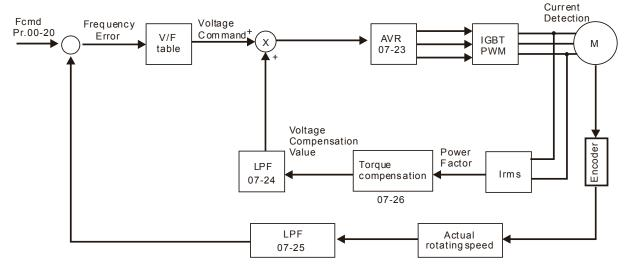
When Pr. 00-10 = 0 and set Pr. 00-11 to 2, the sensorless vector control diagram is shown as follows:
