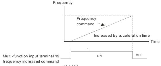
When Pr. 02-09 set to 1: increasing / decreasing frequency command (F) according to the setting of Pr. 02-10 (0.01~1.00 Hz/ms).
