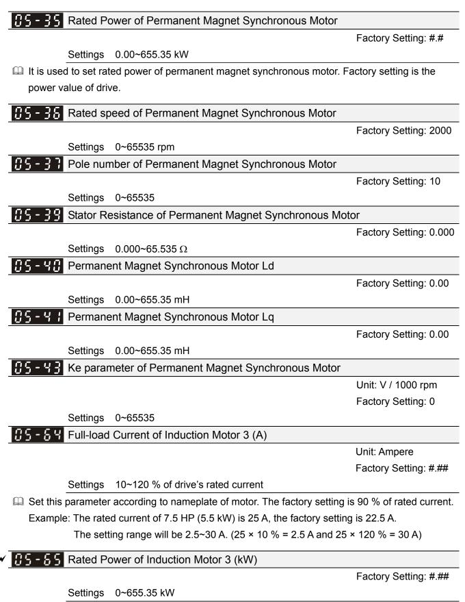
It is used to set rated power of motor 3. Factory setting is the power value of drive.
