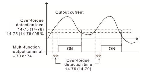
When Pr. 14-74 or Pr. 14-77 setting is 2 or 4, drive will display ot3 / ot4 error when over-torque detection and drive will stop operation, it will operate by manual reset.
