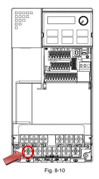
Torque (±10%) Frame D: 20 kg-cm [17.4 lb-in.] [1.96 Nm] Frame E: 25 kg-cm [21.7 lb-in.] [2.45 Nm]
