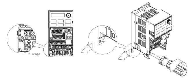
Frame B~F (model with built-in EMC filter)
