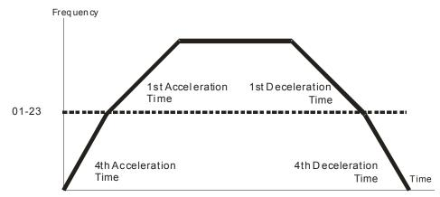
1st/4th Acceleration/Deceleration Frequency Switching
