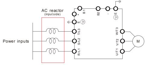
Connecting an AC input reactor
