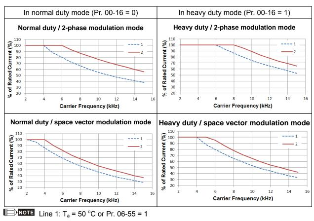
Line 2:  $T_a = 40 \,^{\circ}C$  and Pr. 06-55 = 0/2
