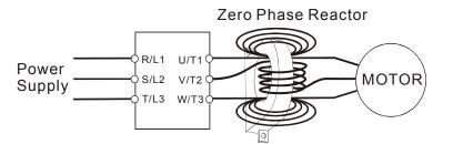
Figure B: Multi-Turn Zero Phase Reactor
