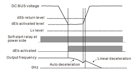
Situation 2: Momentary power loss/ power current too low and unstable/ power supply sliding down because of sudden heavy load
