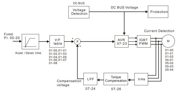
When Pr. 00-10 = 0 and set Pr. 00-11 to 1, the V/F control + encoder diagram is shown as follows:
