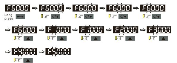
General Mode 2 (maximum operating frequency 01-00 is three digits, e.g.: Pr. 01-00=599.0 Hz)
