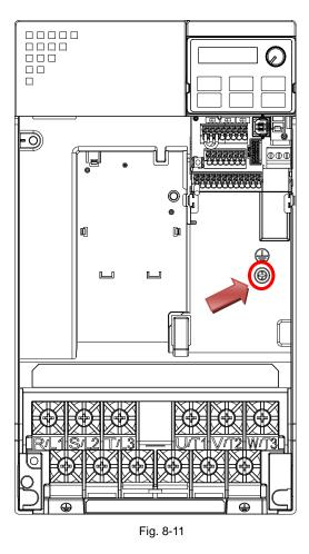
Torque (±10%) Frame F: 7 kg-cm [6.1 lb-in.] [0.69 Nm]
