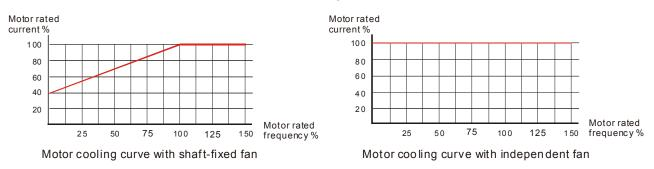
The action of electronic thermal relay depends on the setting of Pr. 06-13 and Pr. 06-27.
