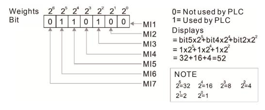
**G2-53** Display External Multi-function Output Terminal Occupied by PLC
