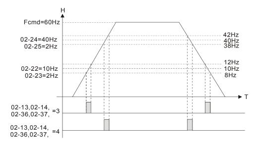
✓ 32-34 Output Frequency Setting for Multi-function Output Terminal
