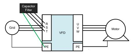
Capacitive filter and drive wiring figure :
