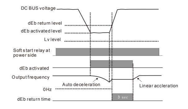
• Situation 3: Power supply unexpected shut down / power loss
