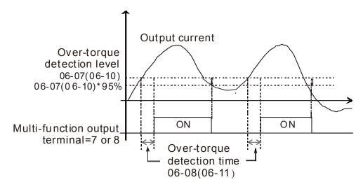
When Pr. 06-06 or Pr. 06-09 is set to 2 or 4, there will be ot1 / ot2 warning displayed and the drive will stop running after over-torque detection. The drive will keep running after manually reset.
