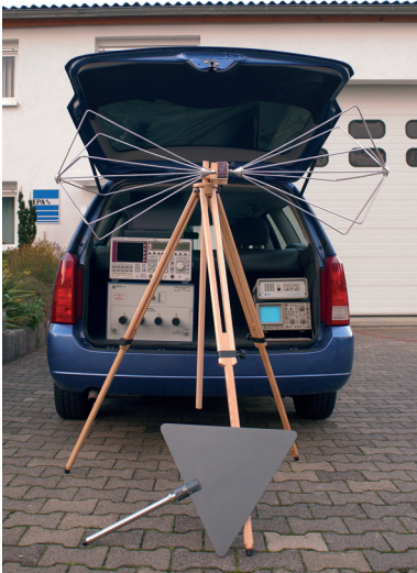
Mobile EMV-Messausrüstung Mobile EMC test equipment
